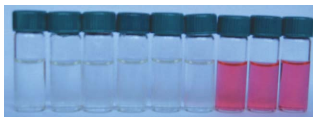
Fig. 3 The color change of 2 in pH 7.40 of phosphate buffer solution (MeOH–H 2 O = 3:7, v/v) in the presence of 10 equiv. of certain amino acids. From left to right: none, Tyr, Glu, Met, Lys, His, Cys, Hcy and GSH. [ 2 ] = 2.0 \times 10^{-5} M.
